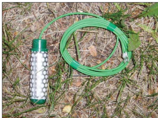
Granular matrix sensor. NCAT photo.
