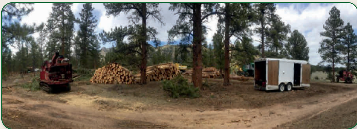
Landing and harvesting equipment where the trees are sized, sorted, processed, and loaded out.
